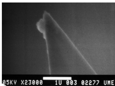
Figure 2. SEM image of carbon build up on a tip. The thickness of this coating is on the order of 50 nm, and there is evidence of carbon loading as far as 1 \mu\text{m} from the apex of the tip.
